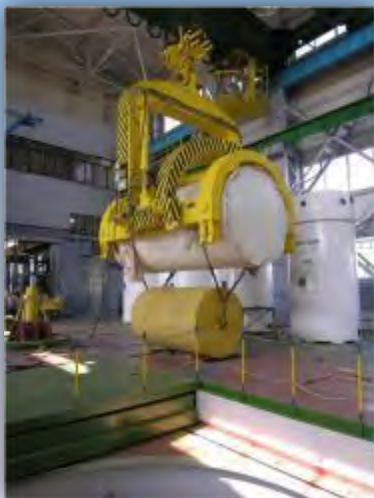
Transfer and packing cask and railway carrier to transport SNF for storage
