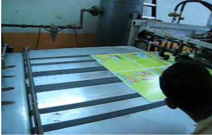
UV curing process of overprint varnishes (OPV)
